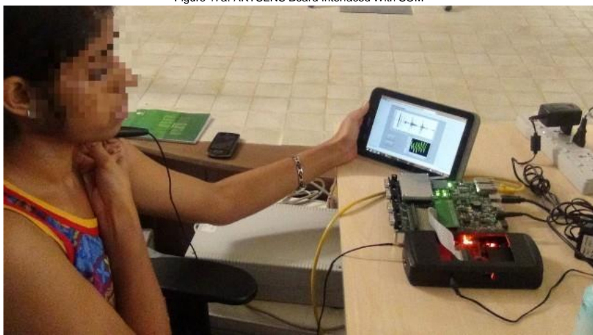
Figure 17b. Stiffness Measurements Performed In-Vivo Using ARTSENS Implemented With SOM
